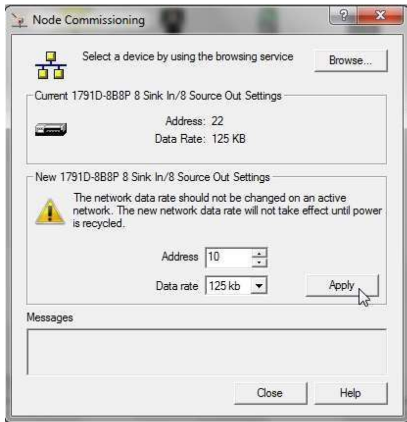
Figure 11-A Modified Address Node Commissioning Window
